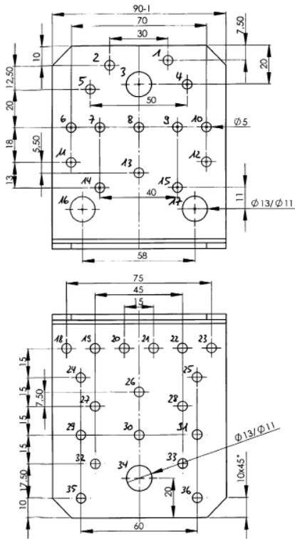
Figure B. 5 Dimensions of Angle Bracket 89 552
