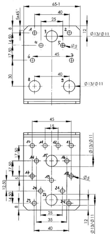
Figure B. 3 Dimensions of Angle Bracket 89 550
