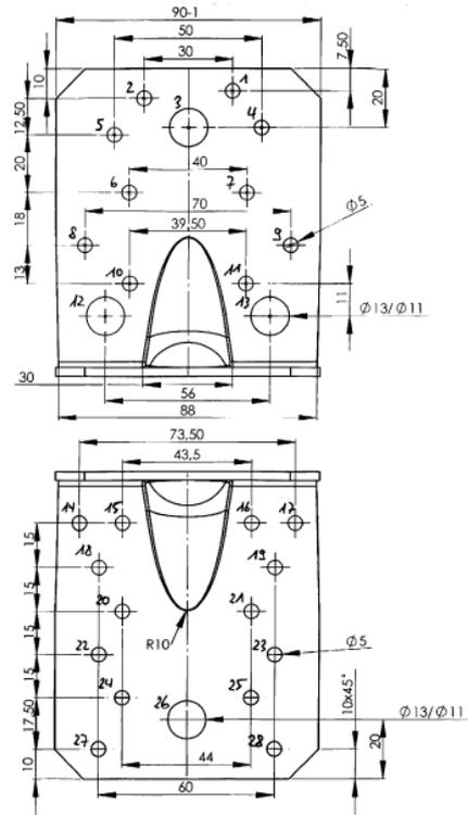
Figure B. 6 Dimensions of Angle Bracket 89 553
