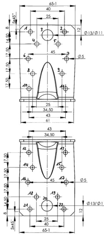
Figure B. 4 Dimensions of Angle Bracket 89 551
