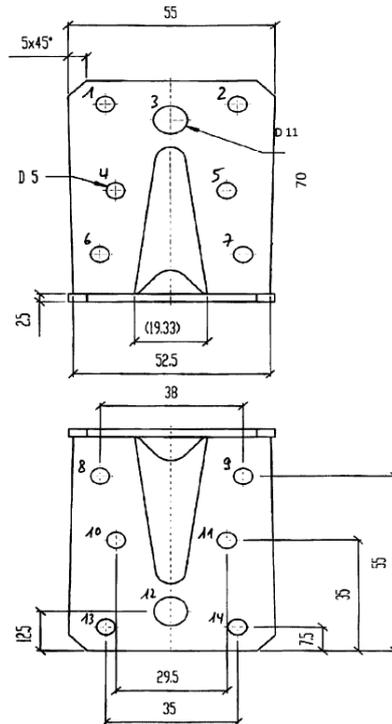
Figure B. 2 Dimensions of Angle Bracket 89 541
