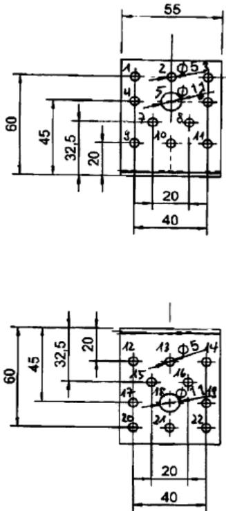
Figure B. 1 Dimensions of Angle Bracket 89 540
